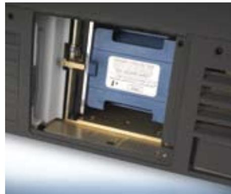
▲ User-replaceable Xenon lamp modules with adjustable lamp power for lower brightness.
