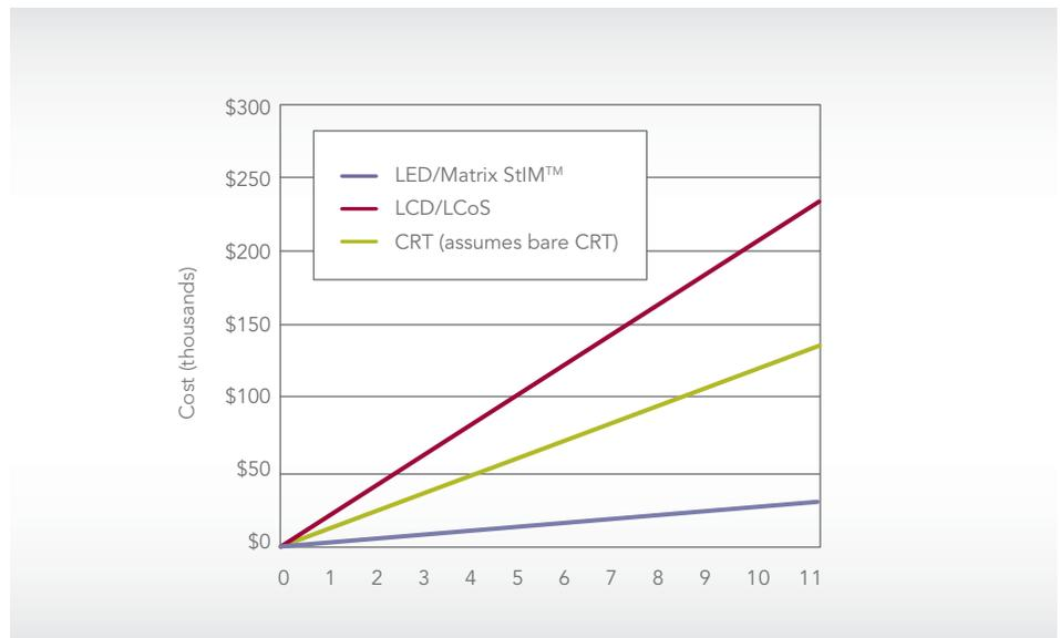
▲ With 50,000 hours MTBF on the illumination package, no moving parts, no lamps or filters to change, operation is virtually maintenance-free. High MTBF and ease of support contribute to a noticeably low cost of ownership and savings in sustainment costs.
