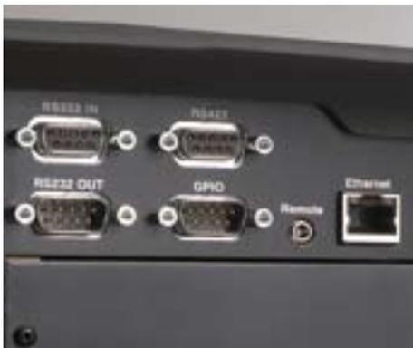
▲ The widest source compatibility – includes built-in Ethernet networking for full compatibility for projector monitoring and control capabilities.
